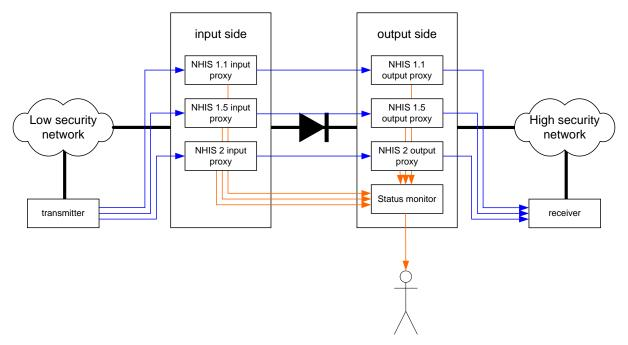
The diode terminates NHIS streams on the input side, acting as a standardscompliant NHIS receiver. The NHIS streams transit the one-way network in an internal representation of the NHIS PDUs and are reconstructed on its output. The diode must act as an NHIS compliant sender on the output side.
