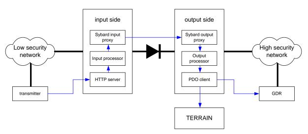
The system is pictured in detail above. The system consists of two nodes connected by a one-way optical network. The one-way network is managed by the Sybard diode product which manages the delivery of files over the diode network.
