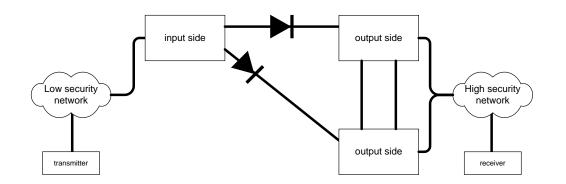
Failure of the diode input side does not result in data loss for NHIS delivery, as the NHIS protocol includes features which provide resilience against data loss.
