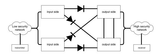
The increased resilience of this configuration would considerably reduce the risk of failure, and thus reduce data loss. A fully redundant diode may be expensive: a cheaper configuration might be introduced by removing the redundancy of the input side:
