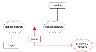
The probe is likely not integrated with the ISP network, and so must deduce the presence of a target's communications by studying the protocols which make up the
