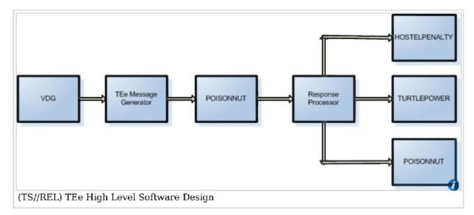
(TS//REL) The TEe takes in CollectionSessions from VDG and sends all IKE and ESP to POISONNUT. When a response comes back from POISONNUT, the associated File is then decrypted. The decrypt is sent to TURTLEPOWER
