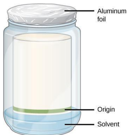
Figure 10.4: Chromatography can be set up in a container such as a Mason jar. The start line of the sample, the origin, is shown above the solvent.
