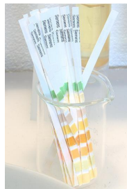
Figure 7.2: Diastix glucose detection strips turn from blue to green to yellow to brown with increasing concentrations of glucose.
