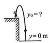
(a) Knowns: t = 2.35 s; y = 0 m;  $v_0 = +8.00 \text{ m/s}$ ;  $a = -9.8 \text{ m/s}^2$
