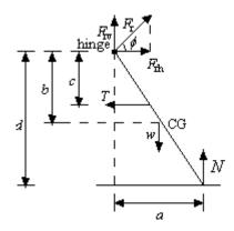
$$a = \frac{1.10}{2} = 0.550 \text{ m}, b = \frac{1.30 \text{ m}}{2} = 0.650 \text{ m}, c = 0.500 \text{ m}, d = 1.30 \text{ m},$$
