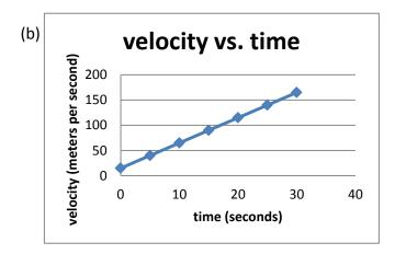
In the velocity vs. time graph, we can identify two points:  $v=65~\mathrm{m/s}$ ,  $t=10~\mathrm{s}$  and  $v=140~\mathrm{m/s}$ ,  $t=25~\mathrm{s}$ . Therefore , the slope is  $a=\frac{\mathrm{rise}}{\mathrm{run}}=\frac{(140-65)~\mathrm{m/s}}{(25-10)~\mathrm{s}}=5.0~\mathrm{m/s}^2$
