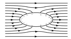
The field lines deviate from their original horizontal direction because the charges within the object rearrange. The field lines will come into the object perpendicular to the surface and will leave the other side of the object perpendicular to the surface.
