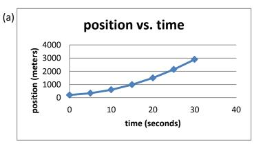
In the position vs. time graph, if we draw a tangent to the curve at  $t=20\,\mathrm{s}$ , we can identify two points:  $x=0\,\mathrm{m}, t=5\,\mathrm{s}$  and  $x=1500\,\mathrm{m}, t=20\,\mathrm{s}$  so we can calculate an approximate slope:  $v=\frac{\mathrm{rise}}{\mathrm{run}}=\frac{(2138-988)\,\mathrm{m}}{(25-15)\,\mathrm{s}}=115\,\mathrm{m/s}$
